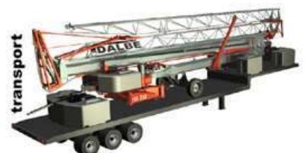
gru e zavorra completa su 1 camion crane and complete ballast on 1 truck
